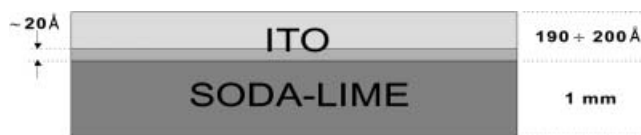
Figure 4. Bruggman effective medium approximation (BEMA) model of the Balzers ITO-coated glass substrates. The ITO films were modelled by the superposition of two layers, each described by a combination of N Lorentz oscillators.
